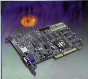
The Voodoo4 4500 (pictured above) and Voodoo5 5000 will both come in a PCI flavor.
